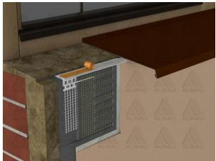
Application: Self-adhesive under sill PVC profile 90° with glass fibre mesh and self-adhesive foam tape is used to make safe and dense expansion jointing between the window sill and insulation system ETICS. Profile protects insulation system against mechanical damage and ensures water draining in vertical direction from the system. Glass fibre mesh meet the ETAG 004 requirements. Comply with ETICS insulation system
